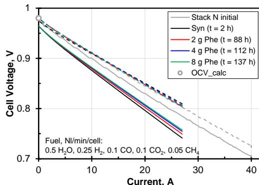
Figure 6: I-V-curves of Stack P on syngas plus 0, 2, 4 and 8 g/Nm<sup>3</sup> of phenol together with data from Stack N.  $T_{\text{stack}} = 700\text{ }^{\circ}\text{C}$ . Data for Stack P was fitted with a hyperbolic plus linear term for better visibility.
