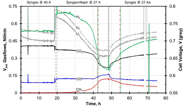
Figure 4: Flow rate of main gas components CO, CO<sub>2</sub>, CH<sub>4</sub> and H<sub>2</sub> in the anode exhaust gas during measurement at Stack N.  $U_1$  voltage of lower cell and  $U_2$  voltage of upper cell.  $T_{\text{stack}} = 700^\circ\text{C}$ .
