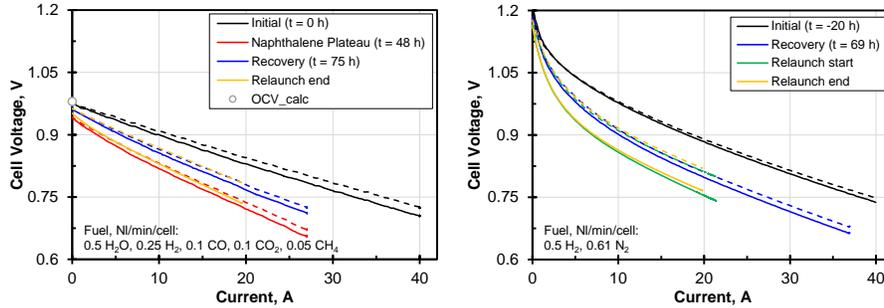
Figure 3: Left: I-V-curves of Stack N on syngas at indicated instants. Right: I-V-curves on  $H_2/N_2$  mixture at indicated instants. Solid lines represent voltage of lower cell.  $T_{stack} = 700$  °C. Noisy data were fitted with a hyperbolic plus linear term for better visibility.
